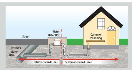
As shown in the above diagram, two sections of the water service line need to be inventoried: Utility (District) Owned: The line that runs from the water main to the water meter. Customer Owned: The line that runs from the water meter to your home.
