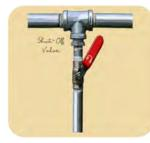
If you have a valve near where the leak is, or a shutoff valve inside your house where the water service line enters the house, turn the valve off. This will stop water from leaking until you can arrange for a plumber to do a repair or for you to do the repair yourself.
